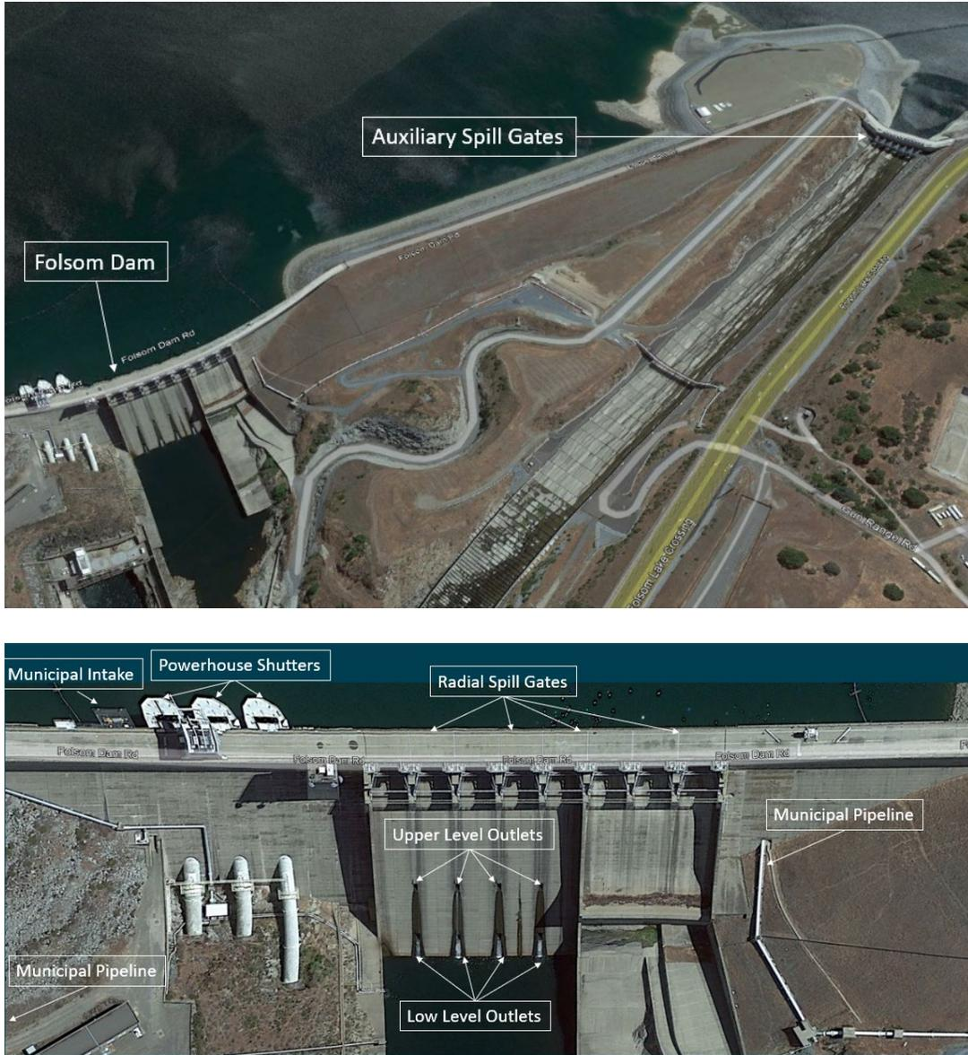
Figure 5-23. Folsom Dam and Auxiliary Spillway (top) and Folsom Dam (bottom).
