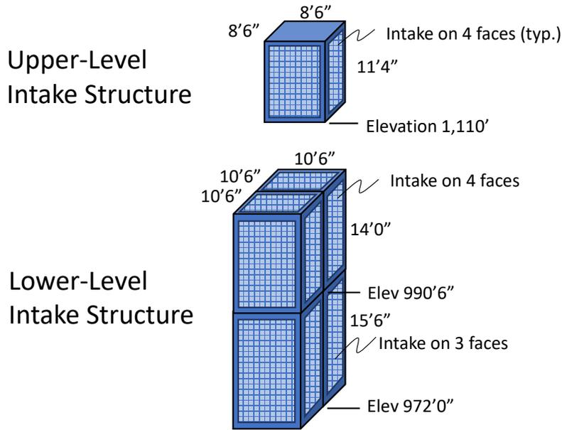
Figure 5-19. Schematic of upper-level (top) and lower-level (bottom) Whiskeytown Dam intake structures.
