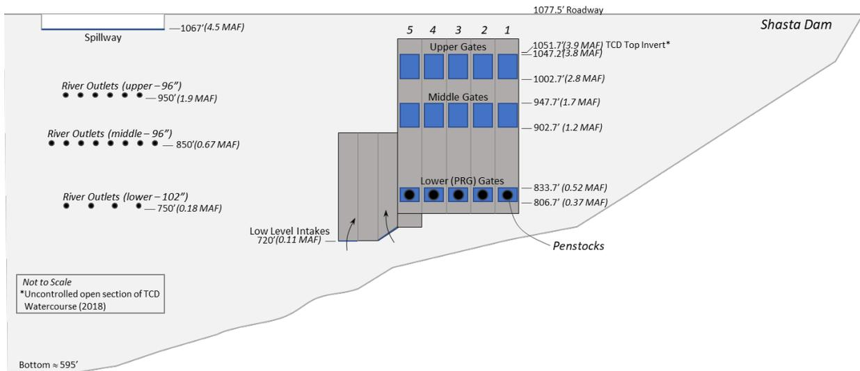
Figure 5-3. Shasta Dam outlet works and Temperature Control Device, view looking downstream at upstream face of dam. Powerhouse units 1 through 5 are shown for reference.
