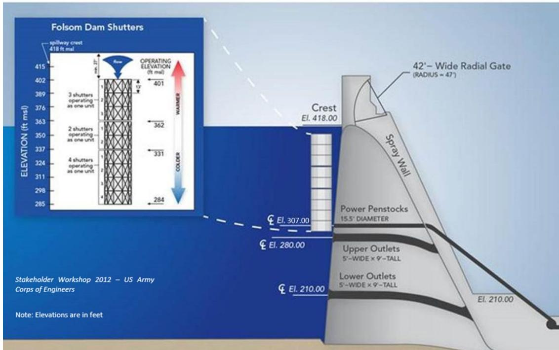
Figure 5-26. Side View Schematic of Folsom Dam Outlets and Shutters.
