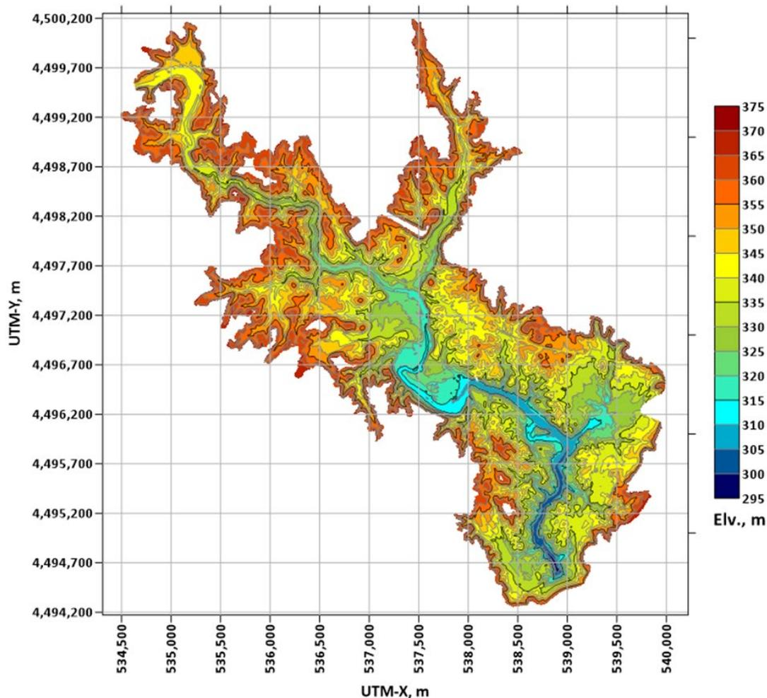
Figure D-2. Whiskeytown Lake bathymetry map with the data collected during May 2019 SWATHPlus survey of Whiskeytown Lake, California. 2-meter (6.56-feet) resolution.
