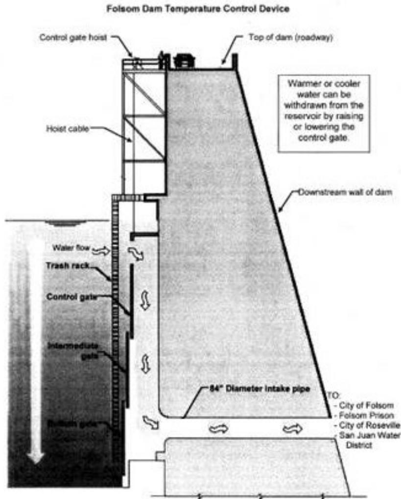
Figure 5-25. Folsom Dam side-view with Municipal Water Supply Intake Structure Illustration.
