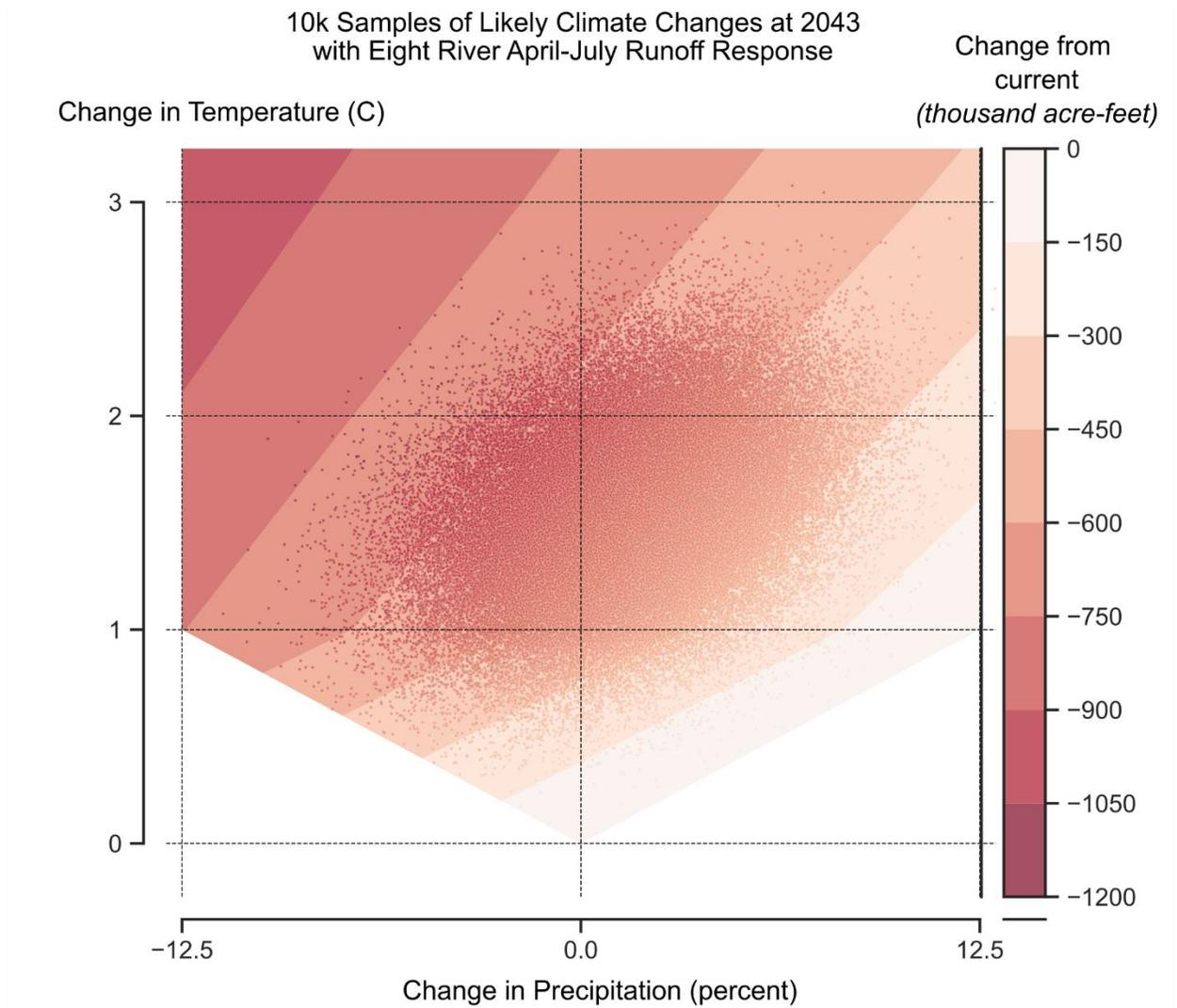
**Figure 5-15 Cumulative Distribution Function of System Performance Across Model Ensemble-Informed Climate Uncertainty Space at 2043 (using Eight River Index April-to-July Response Surface)**
