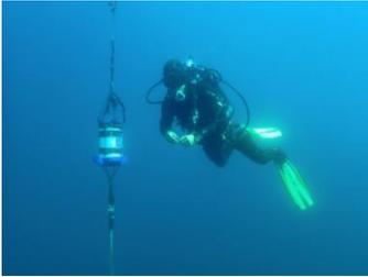
*UC Davis field technician deploying an Acoustic Doppler Current Profiler to measure water velocities in Lake Tahoe in a similar fashion that will be deployed in this study.*
