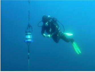
*UC Davis field technician deploying an Acoustic Doppler Current Profiler to measure water velocities in Lake Tahoe in a similar fashion that will be deployed in this study.*
