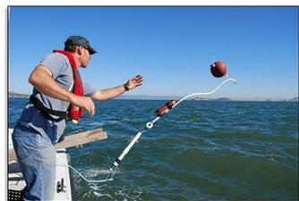
*Arnold Ammann deploying an acoustic receiver under the Golden Gate Bridge.*
