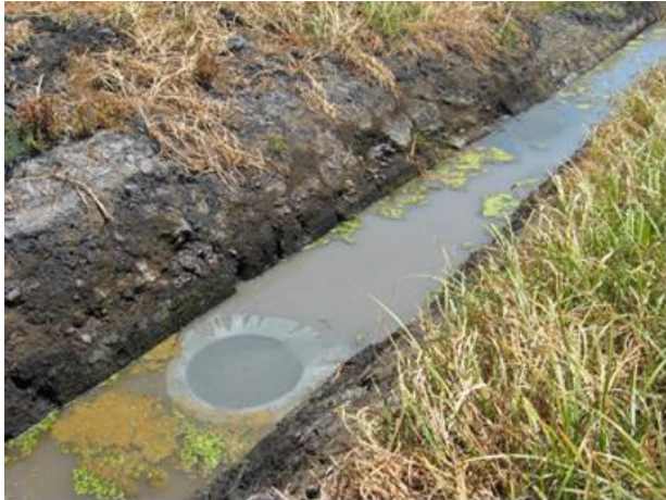
Figure 4. Active boil on Jones Tract observed in 2011. Photo credit: Gerald Bawden
