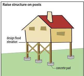
**Figure 7-8** | Floodproofing in accordance with the National Flood Insurance Program can be achieved through several methods. The illustration on the left shows an example of floodproofing by constructing the lowest floor within a structure above the design flood elevation. The illustration on the right shows floodproofing by raising the bottom of the structure above the design flood elevation.
