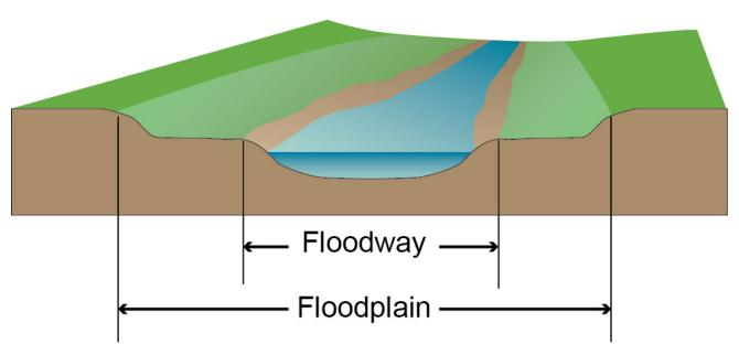
Conceptual Diagram of a Floodway within a Floodplain
