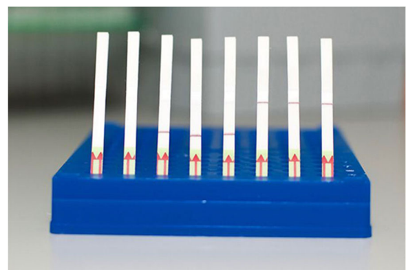
Figure 10. Photograph of SHERLOCK technology applied using test strips which visually indicate genetic identification by the presence or absence of a line on each test strip (Photo Credit: Zhang lab, Broad Institute of MIT and Harvard, Broadinstitute.org).
