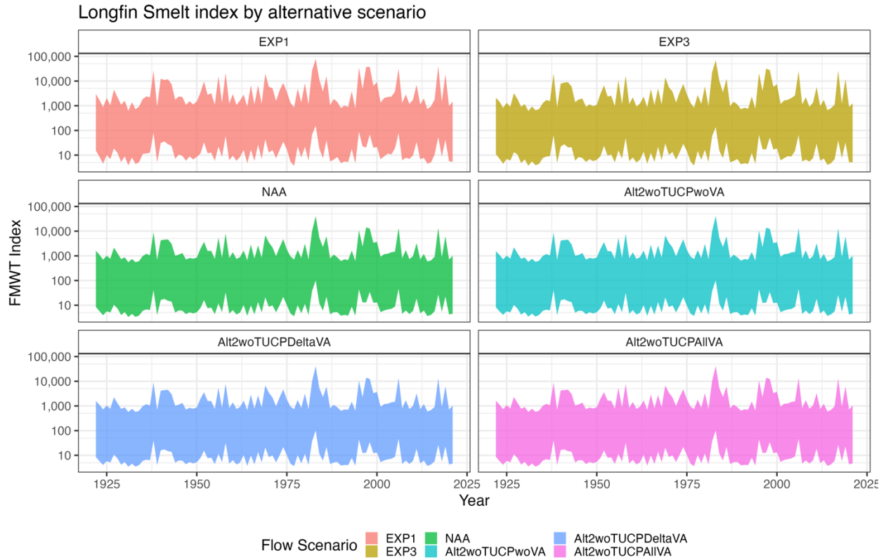
Fig J.1-5. The 95th Bayesian credible intervals for the posterior predictive distributions are shown, based on the parental stock model and the 100 year time series of CalSim 3 Delta Outflow values for each scenario.
